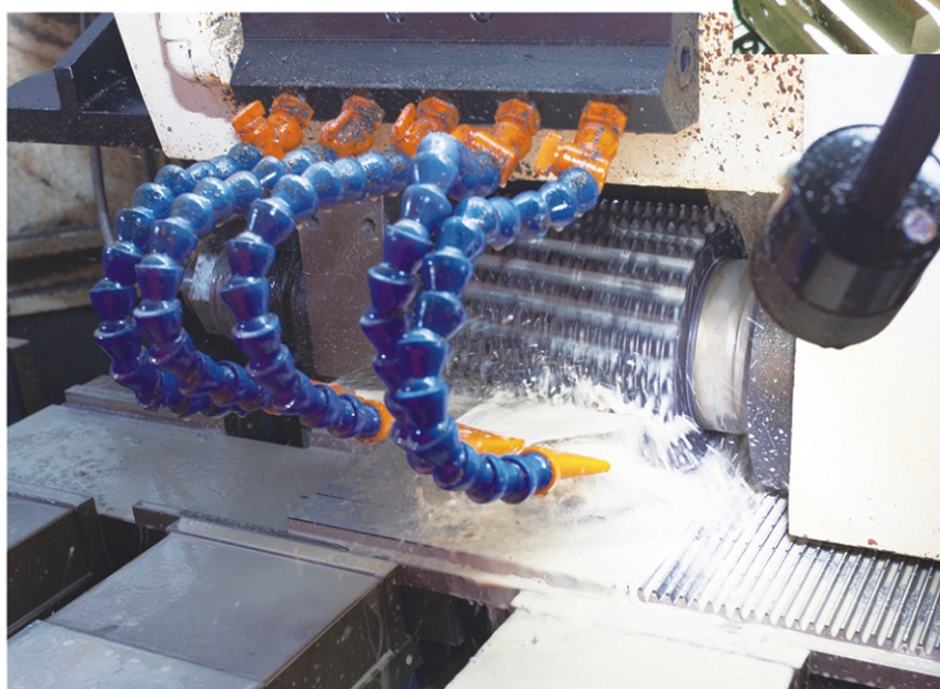
● 齒條滾齒 Milling the rack tooth
